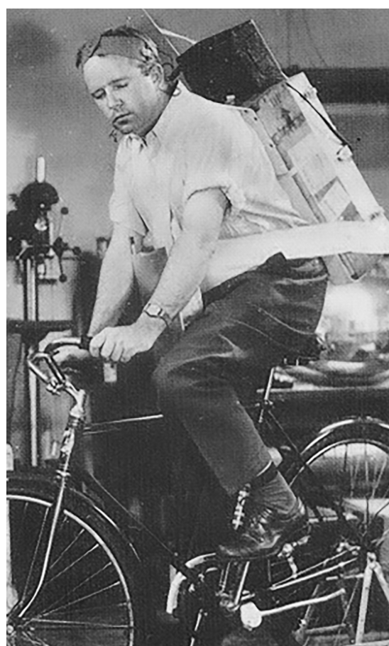
Fig. 2. The original Holter biotelemetric apparatus, manufactured in 1947. It was used to broadcast electroencephalograms and electrocardiograms using coarse heavy battery equipment of almost 40 kg [1]
